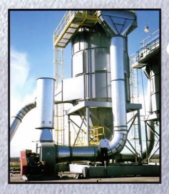
Compressed-air baghouses also cling to their elevated status among elevator operators, often favored because they operate on a small percentage of available plant compressed air. The pair of Aircon 12'-0" diameter compressed-air round baghouses (CAR 193-10) [above] and the larger 14'-0" diameter unit on their side (CAR 276-12) [above left & above right] have no internal fan motor requirements.
